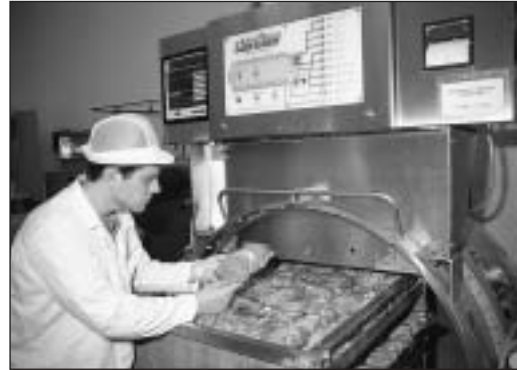
▲ The Barriquand Steriflow retort used in commercial sous vide preparation.
